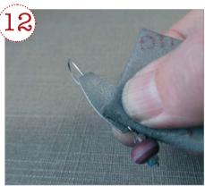
Check that the two earring wires are the same length, both at the long end that will form the earwire itself and at the short end which will form the hook. Trim as necessary and file all four wire ends smooth.
